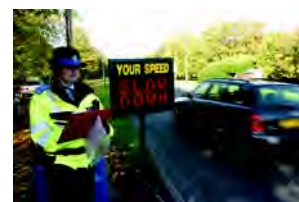
PCSO Using a SID to monitor speed levels
